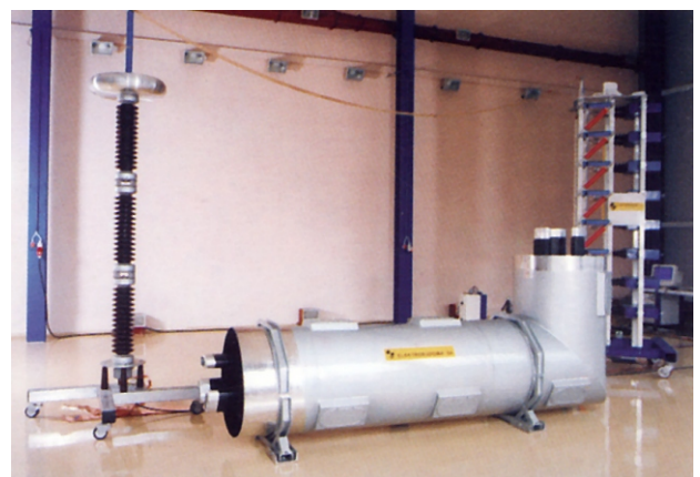
Vista parcial del laboratorio de ensayos Testing the busducts in the Company's high-voltage laboratory
